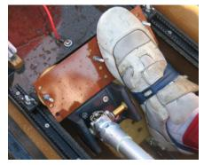
Modified stretcher to enable a para rower with a below knee amputation to use a sliding seat. For safety the prosthesis easily disengages from the footplate in the event of a capsize.
