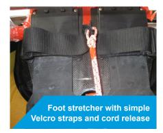
For para rowers who have little or no lower limb function, a footplate with nylon heel cups is used. The Velcro straps can be released using a simple cord release, which when pulled by the athlete ensures that they can release their feet in the event of a capsize.
